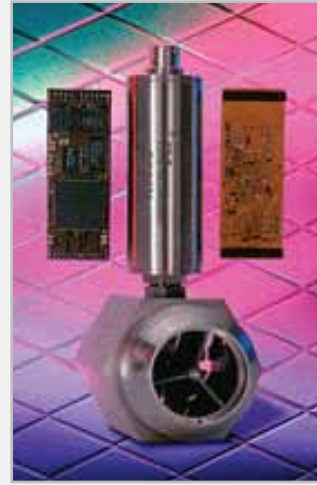
Figure 4. New smart turbine flowmeters incorporate an integrally-mounted electronics package that performs all temperature compensation internally
